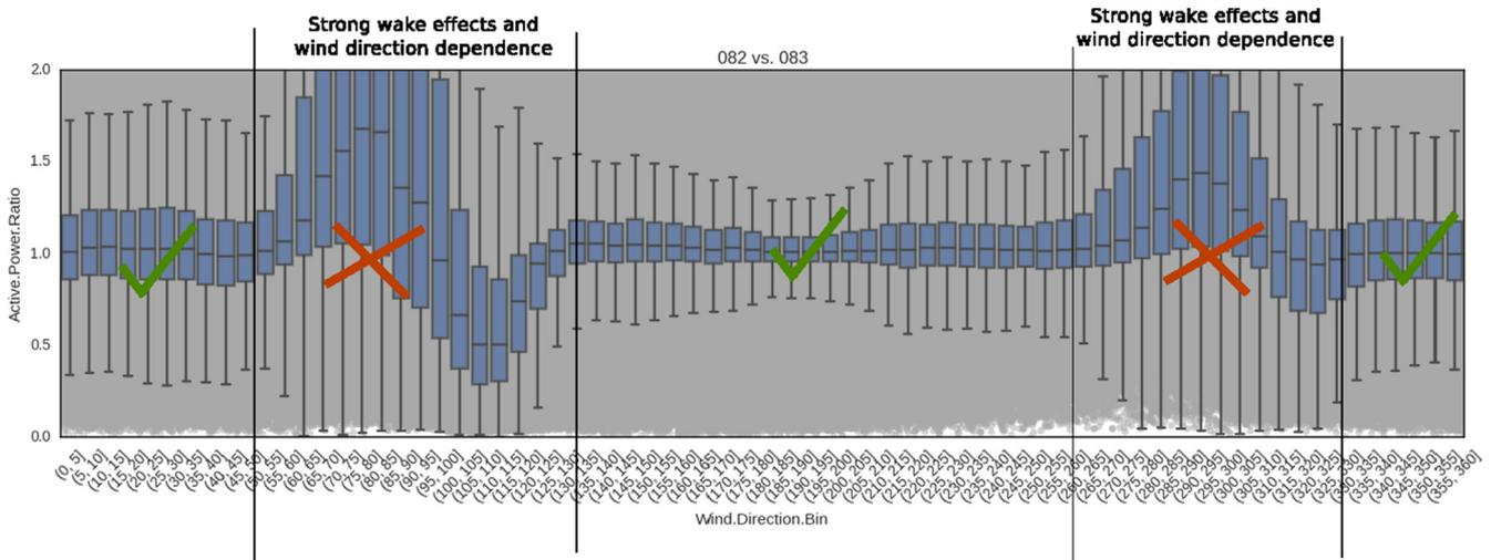
Fig. 1. Identify the wake free data using the power output ratio.
