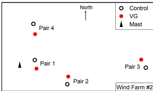
Fig. 4. Layout of the four turbine pairs on wind farm #2. The between-turbine distances are: Pair 1, 3d; Pair 2, 3.3d; Pair 3, 3.3d; and Pair 4, 3.7d. The met mast's distance to the turbine pairs are: Pair 1, 0.2 km, Pair 2, 1.3 km; Pair 3, 3.6 km; and Pair 4, 1.3 km.
