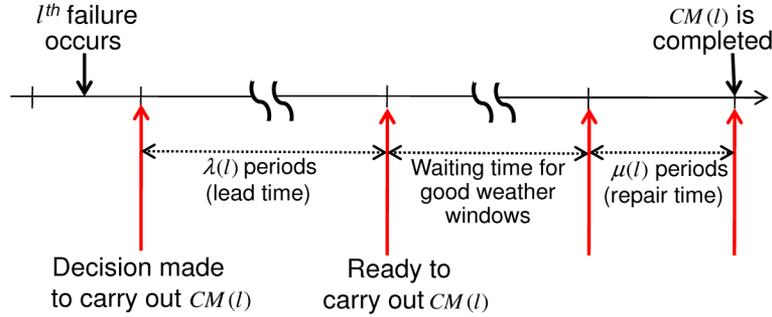
Fig. 3. Corrective maintenance after a failure with the  $l$ th failure mode. The figure illustrates the repairing process after a major failure where  $\mu(l) = 1$ . For a minor failure, the process would be similar except  $\mu(l) = 0$ .
