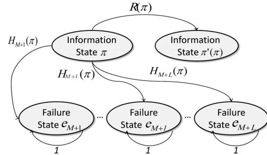
Fig. 2. State transition diagram in the partially observed state space  $S_1$ .
