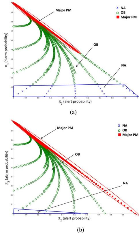
Fig. 8. Optimal decision rule during fall season. (a) In the beginning of fall. (b) At the end of fall.
