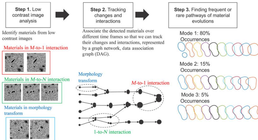
**Figure 5.** Three steps in multi-target tracking analysis of material evolutions and interactions. Step 1 detects individual material objects or structures in noisy images. Step 2 associates the detections from different image frames with each other for estimating the trajectories of material evolutions and interactions. Step 3 finds frequent and rare patterns in the trajectories.
