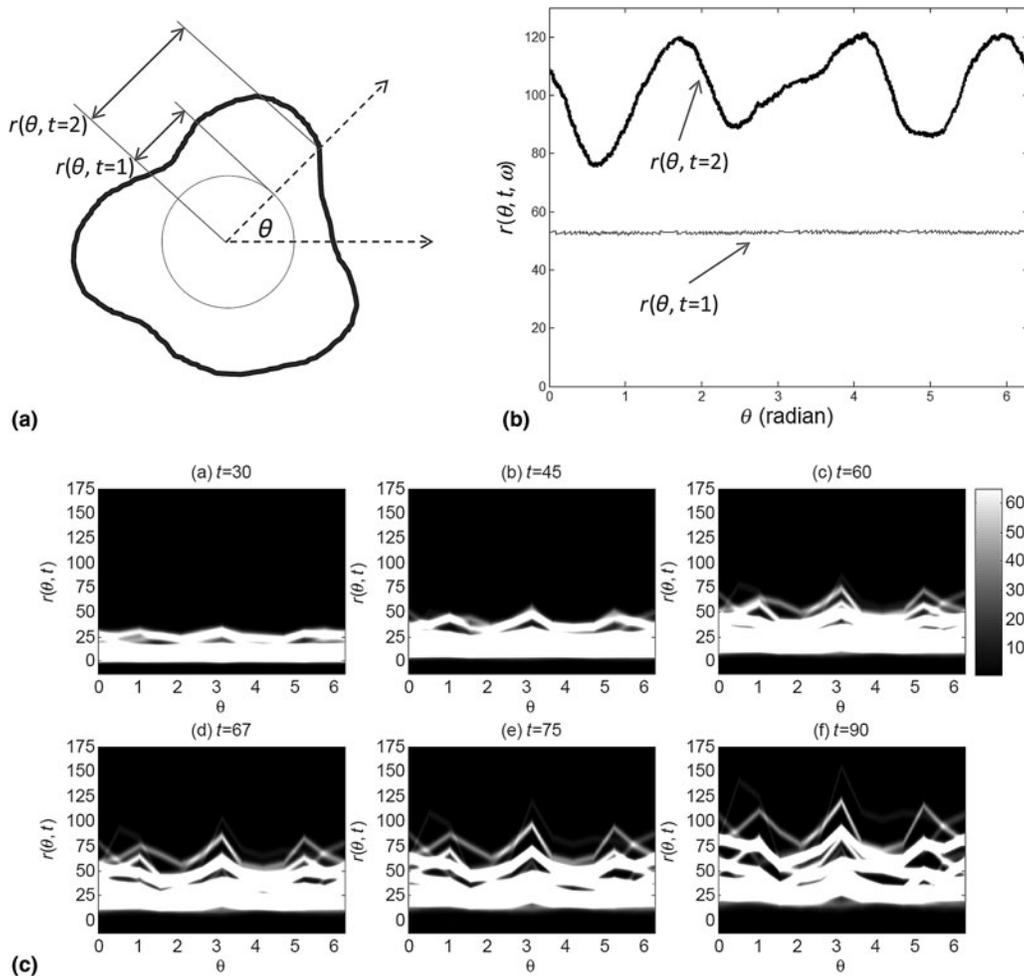
**Figure 4.** Analysis for shape and size evolution of an ensemble of nanoparticles: (a) an outline of material structures in 2d, (b) a curve representation of the outlines, and (c) the variation of material structures represented in terms of the variations of curves and the variations evolve in time. \*Reprinted with permission from Park.<sup>45</sup>
