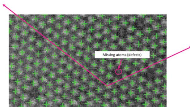
**Figure 3.** Symmetries and defects of atom locations. The crosses point individual atom locations, and two arrow lines represent the basis vectors of a global lattice. \*Figure from Li et al.<sup>30</sup>
