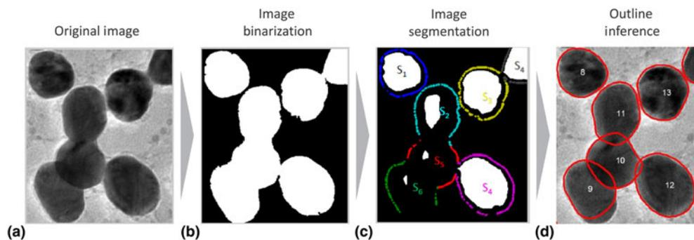
**Figure 2.** (a) Three steps for morphology analysis; (b) the original image is binarized for the binary image of partially overlapping materials in the image; (c) the binary image is segmented into individual foreground images; and (d) the occlusions due to overlaps are estimated and filled for complete outlines. \*Reprinted with permission from Park et al.<sup>21</sup>
