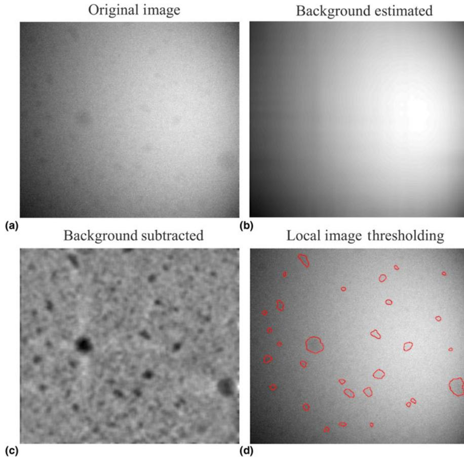
**Figure 1.** Image binarization to extract the outlines of nanocrystals: (a) original image, (b) background image estimated, (c) image after the background subtraction, and (d) outlines extracted by local image thresholding.
